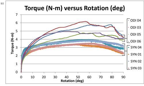
(a) Schematic representation of Talon™ Lag Screw and Helical Blade implantation position as seen in the AP plane and load applied; (b) results of torque to failure testing; (c) graphic depiction of torque to failure testing results. Implants were subjected to a rotation of 1°/sec.
