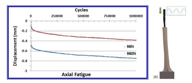
Beyond 1 million cycles (not depicted above) the load was increased 100N every 100,000 cycles for a total of 1.5 million cycles. The final 100,000 cycles was run with a maximum load of 1480N (approximately 332lbs). **The average displacement at 1480N was 3.32mm**. Distal Talons™ were successfully retracted upon completion of the test.
