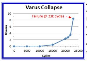
All fluoroscopic images were taken at 100% body weight.  $\alpha_{varus}$  is plotted to the left and illustrated in various x-rays below [E-G]. The lag screw position does not change relative to the femoral head throughout the test.  $\alpha_{neck}$ was <0.1° throughout the test. Nail subsidence was not detected after completion of the test. All Talons™ were successfully retracted after completion of the test.
